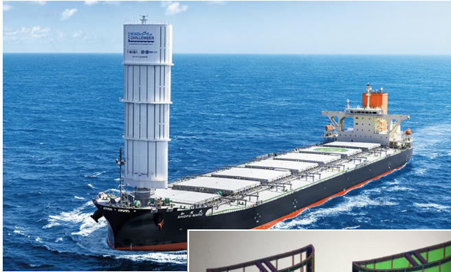
The Wind Challenger: already in service on the bulk carrier »Shofu Maru«
